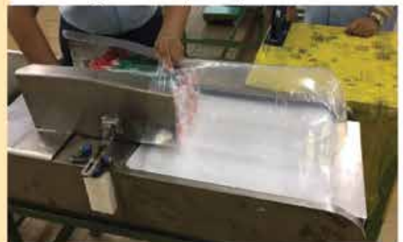
Using Wicket Opening Machine
