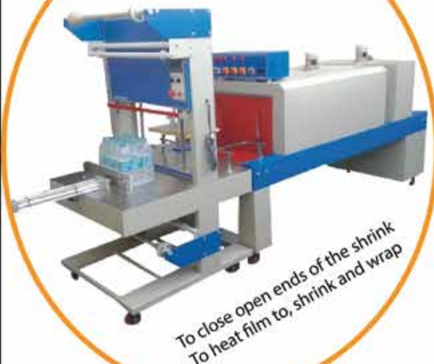
Shrink Wrap Machine used in packaging
